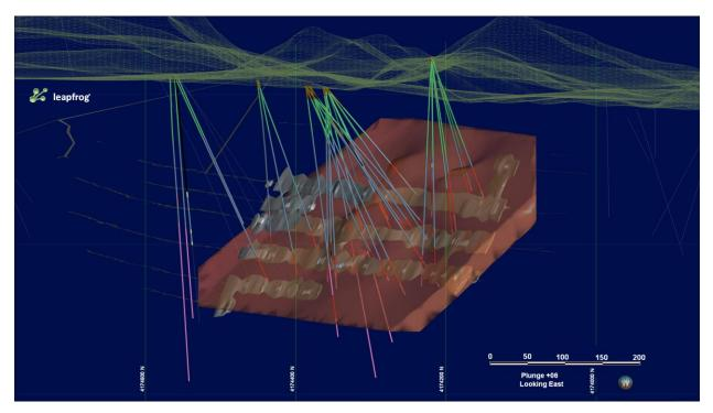
Figure 25 Geological Model of the Nivloc Structure looking east
