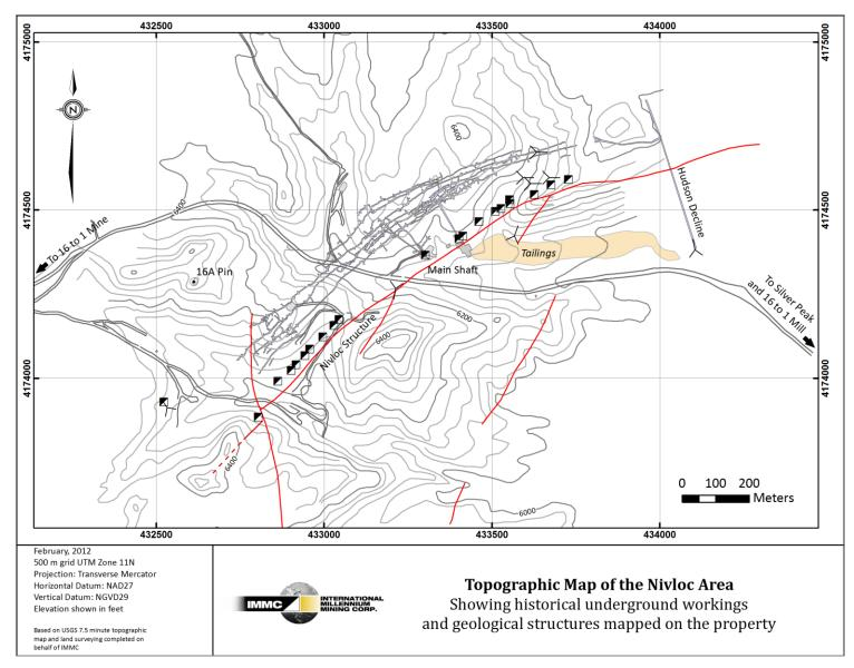
Figure 11 Map of Nivloc Mine Showing topography, shafts and projection of underground workings
