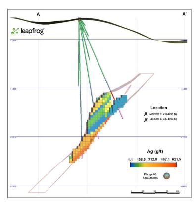
Figure 27 X-section through the southwest part of the Nivloc Target Zone
