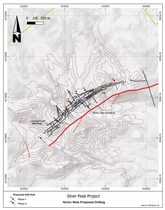
Figure 30 Proposed Drill Holes Nivloc Mine Area
