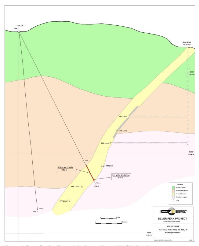
Figure 23 Cross-Section Through the Eastern Part of IMMC Drilled Area
