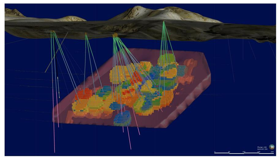
Figure 26 Block Model of the Nivloc Target Zone AgEq Mineralization
